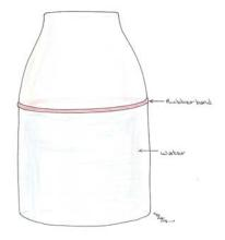
Before you go on you will need a level. You can either use a carpenter's level or you can construct one. To construct a level you will need a small jar half filled with water. While the jar is sitting on a level surface put a rubber band around it at the top of the water. Make sure the rubber band is exactly at the top of the water's surface all the way around the jar.
