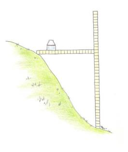
your slope will be 0%. If you are doing this on a slope that is so steep that it is 100 cm from the downhill end of your horizontal meter stick to the ground, you are measuring a 100% slope.
